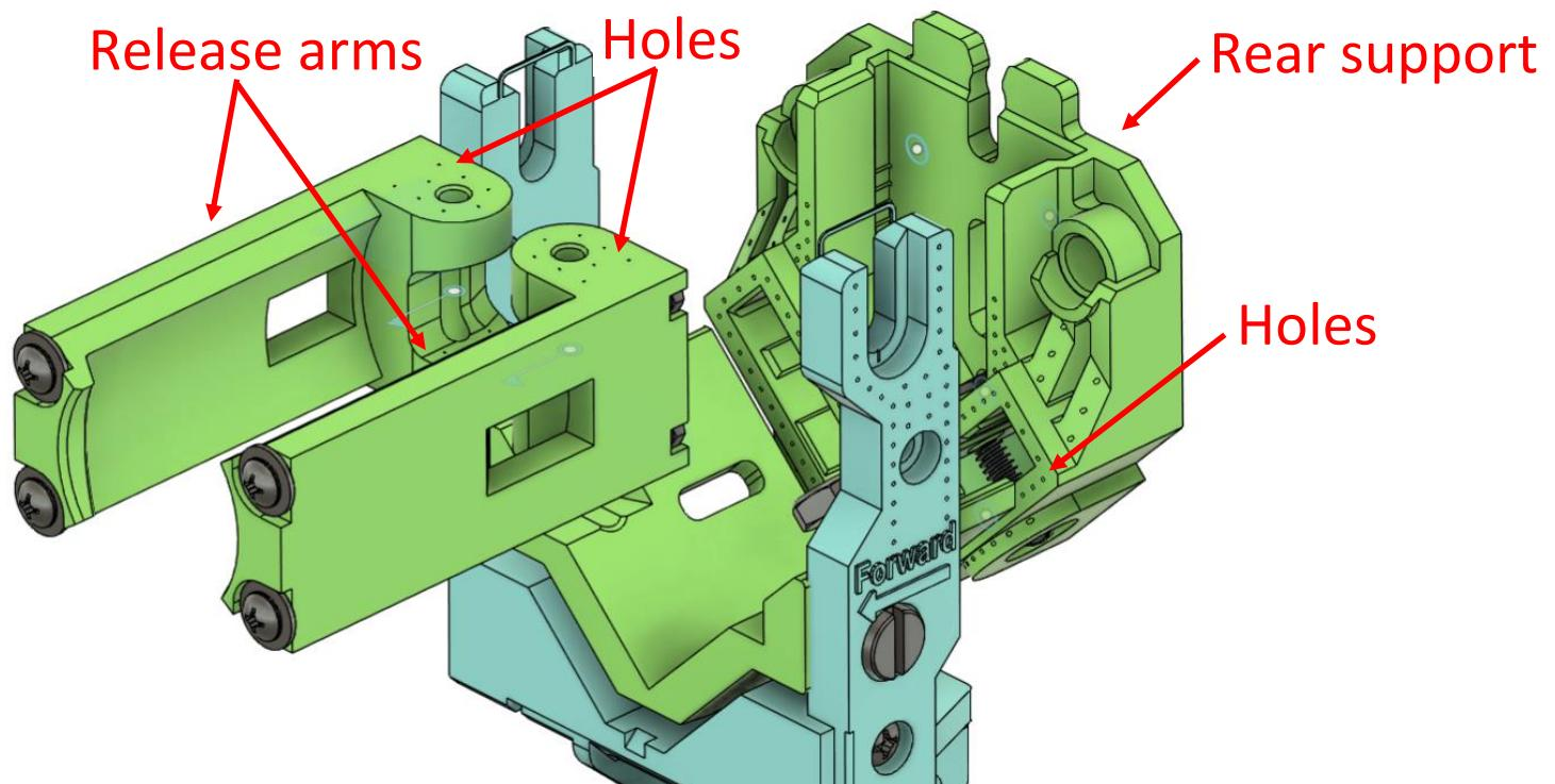
Here is the rear support shown in Fusion and Cura (slice through center of part). Most of the holes surround the pocket, which slides on to the angle that supports the rocket and other components. Forces of the top of the support during launch will impart a moment (torque) that will stress the walls around the angle. There will also be shear forces at the holes of the mounting screws.
