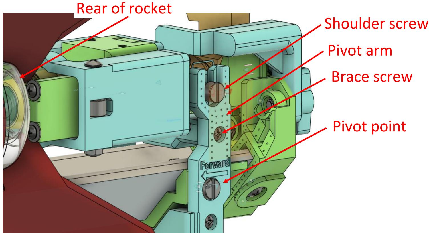
Here is a view with some parts removed. Note the small holes in the **release arms** and in the **rear support**.
