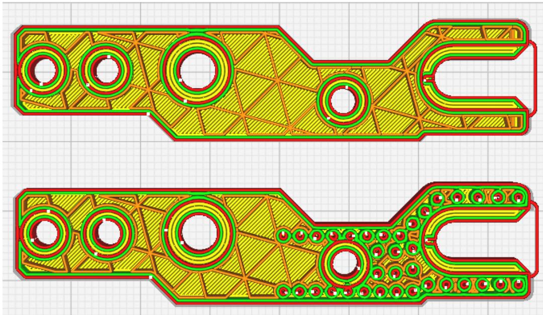
This is a view of the release mechanism of a rocket launcher showing the pivot arm. One can see the small holes around the slot for the shoulder screw and brace screw. Due to required clearances, the pivot arm needs that shape.
