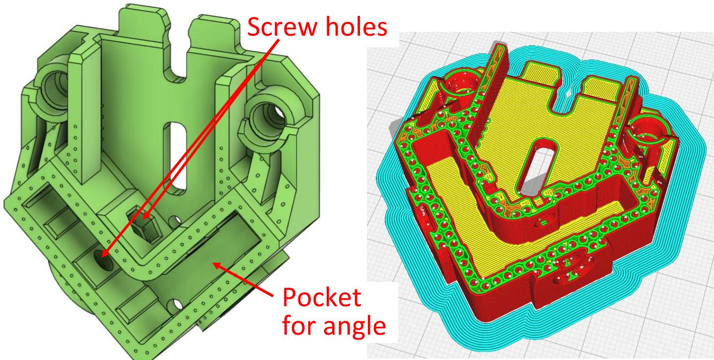
Here is a release arm with holes visible around the pivot shaft hole.
